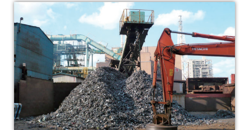
Iron after crushing and sorting of scrap automobiles
